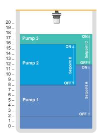
The pump alternation feature of the Vantage 2200 is utilized when the treatment facility has more than two pumps that are to be actuated based upon level set points.
